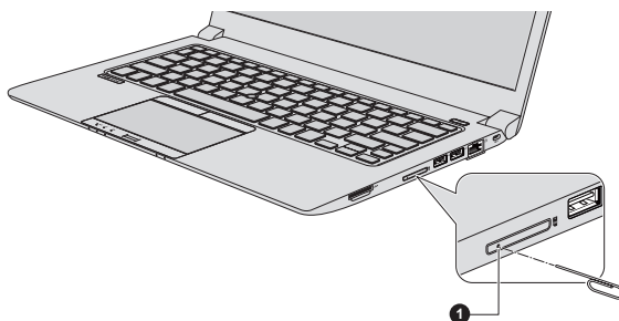
Figure 4-5 Open the SIM card tray with the eject hole (Z40-A)
